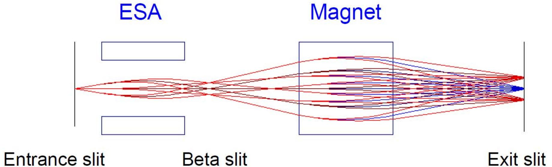
double focusing: ion energies & ion angles
