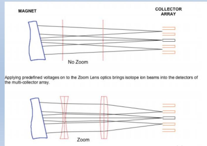
Applying predefined voltages on to the Zoom Lens optics brings isotope ion beams into the detectors of the multi-collector array.
