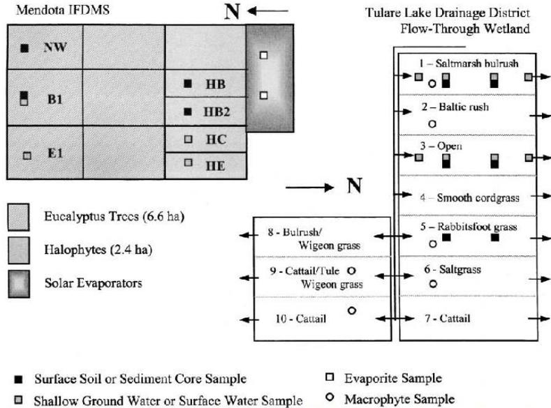
Fig. 2. Integrated on-farm drainage management system (IFDMS) and Tulare Lake Drainage District (TLDD) flow-through wetland generalized designs and sampling locations [after Tanji (1999) and Gao et al. (2000)].
