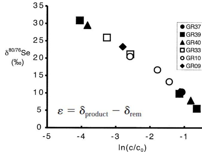
Fig. 4. Se isotope ratio data from all selenate reduction experiments plotted against  $\ln(c/c_0)$ , the natural logarithm of the fraction of unreduced Se remaining. The slope of the line gives  $\varepsilon$ . Uncertainty in  $\ln(c/c_0)$  is approximately the width of the symbols. Uncertainty in  $\delta^{80/76}\text{Se}$  is  $\pm 0.2\text{‰}$ , much smaller than the symbols.
