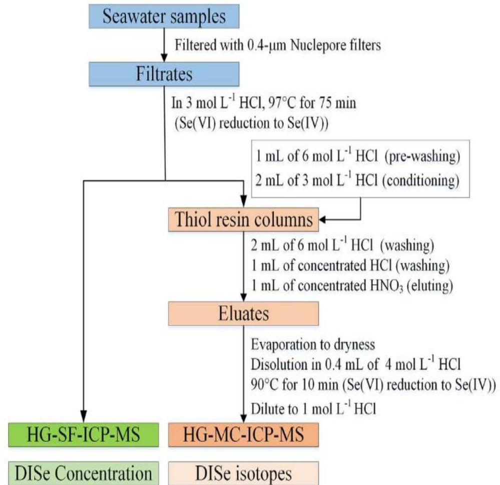
Fig. 1. Analytical procedure for determination of DISE concentration and isotopes in seawater.
